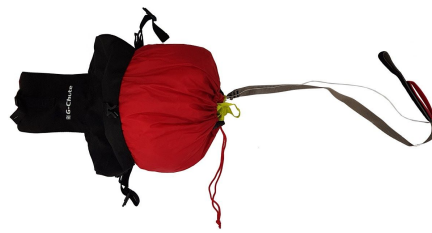
Make sure that there is only a little of the riser visible, while the rest is stored in the red pocket. Close it with the rope.
